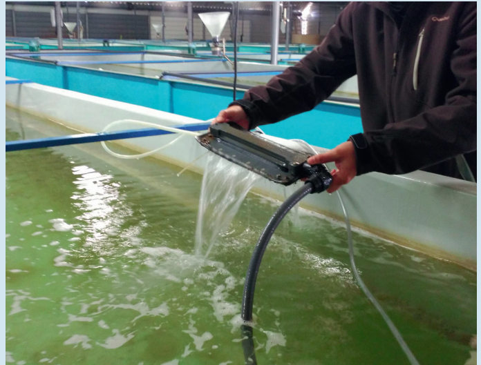
An oxygen aerator that has been developed in the project Aquasef uses microbubbles nozzle technology to achieve efficient and low cost aeration.
