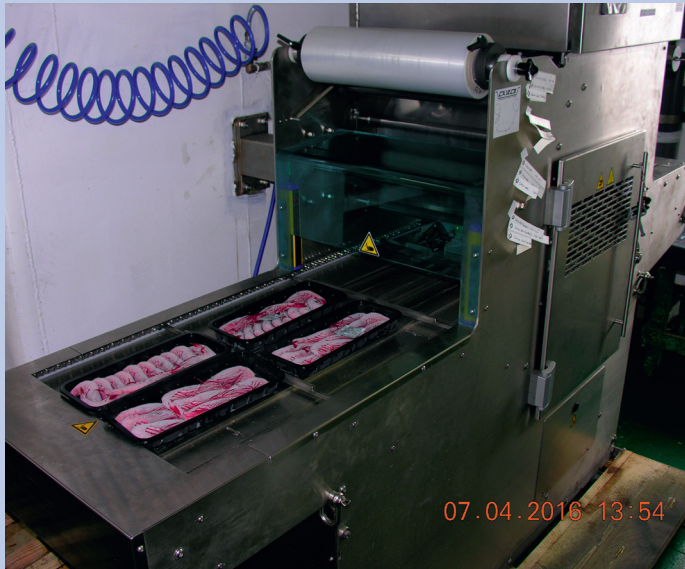
The shrimp samples being processed by the skin packaging machine (a) and the final products (b) ready to be labelled and stored at -18^{\circ}\text{C} .
