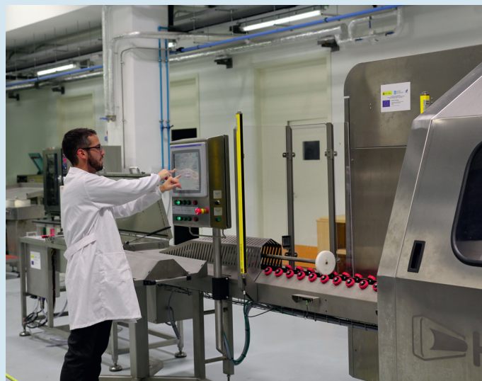
Process Engineer Roberto Carlos Alonso configures the EUR1 million high pressure machine for a test. It can create up to 6000 bars of pressure.
