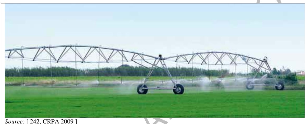
Figure 4.88: Irrigation boom fitted with hanging nozzles to spray slurry-mixed water close to the soil surface
