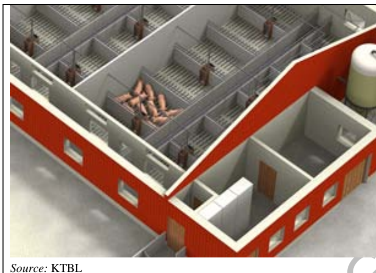
Figure 2.22: Scheme and layout of fully-slatted floored pens in a fattening farm
