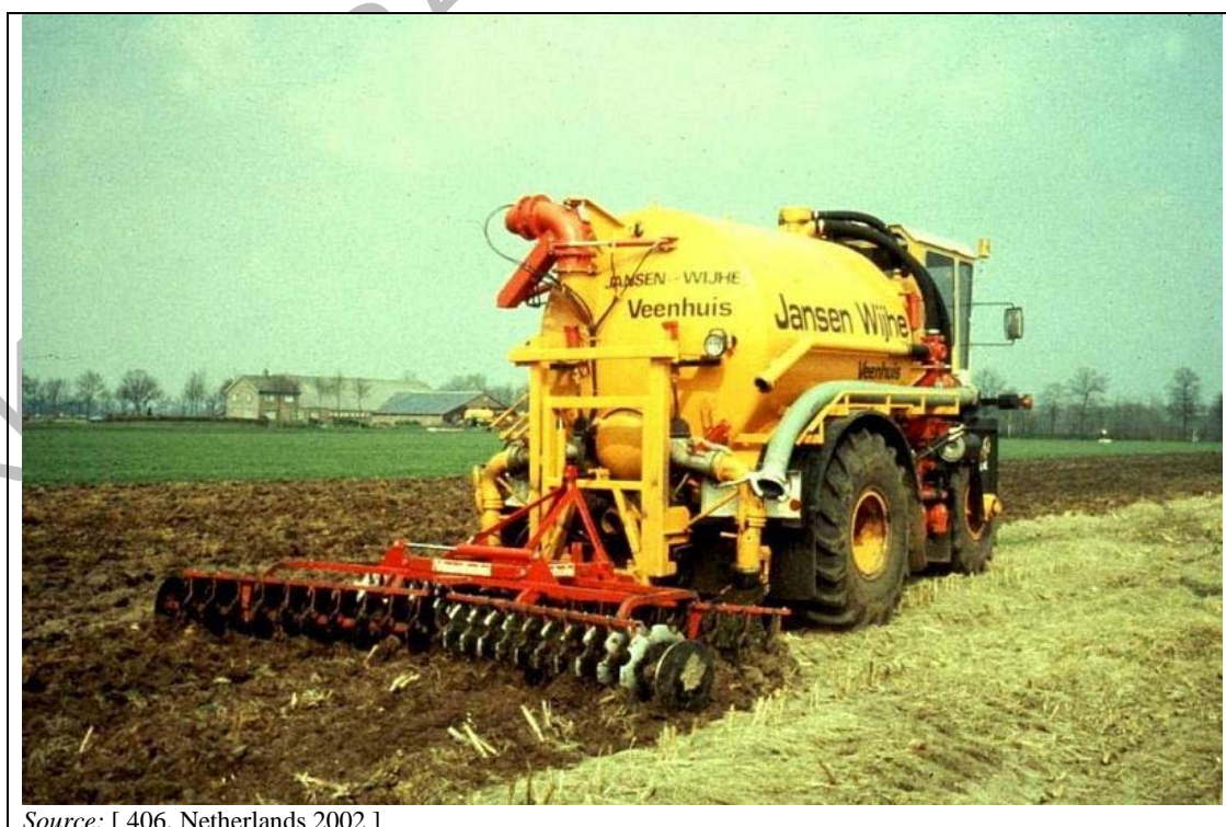
Figure 4.90: Incorporation equipment combined with a big tanker
