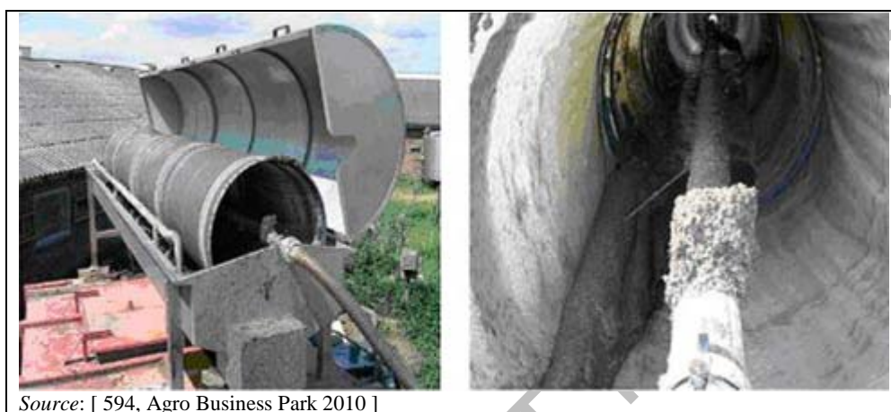
Figure 4.80: Illustration of a rotating (drum) sieve separator for slurry
