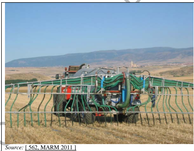
Figure 2.45: Example of a band spreader fitted with rotary distributor to improve lateral distribution
