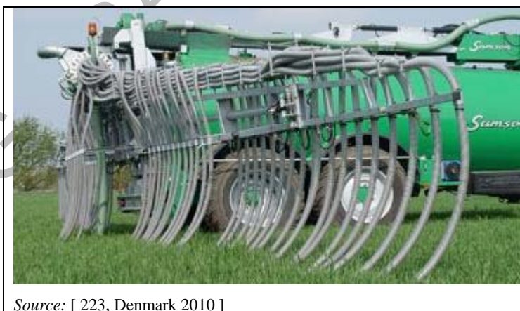
Figure 4.89: Example of trailing hoses mounted on a bar
