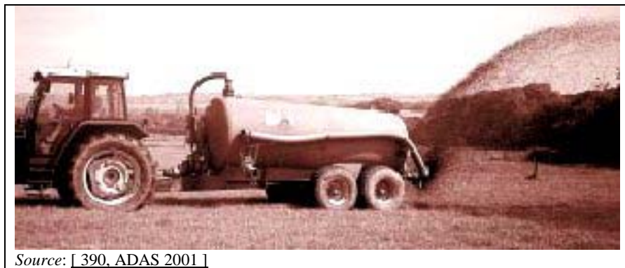
Figure 2.38: Example of a broadcast spreader with a splash plate
