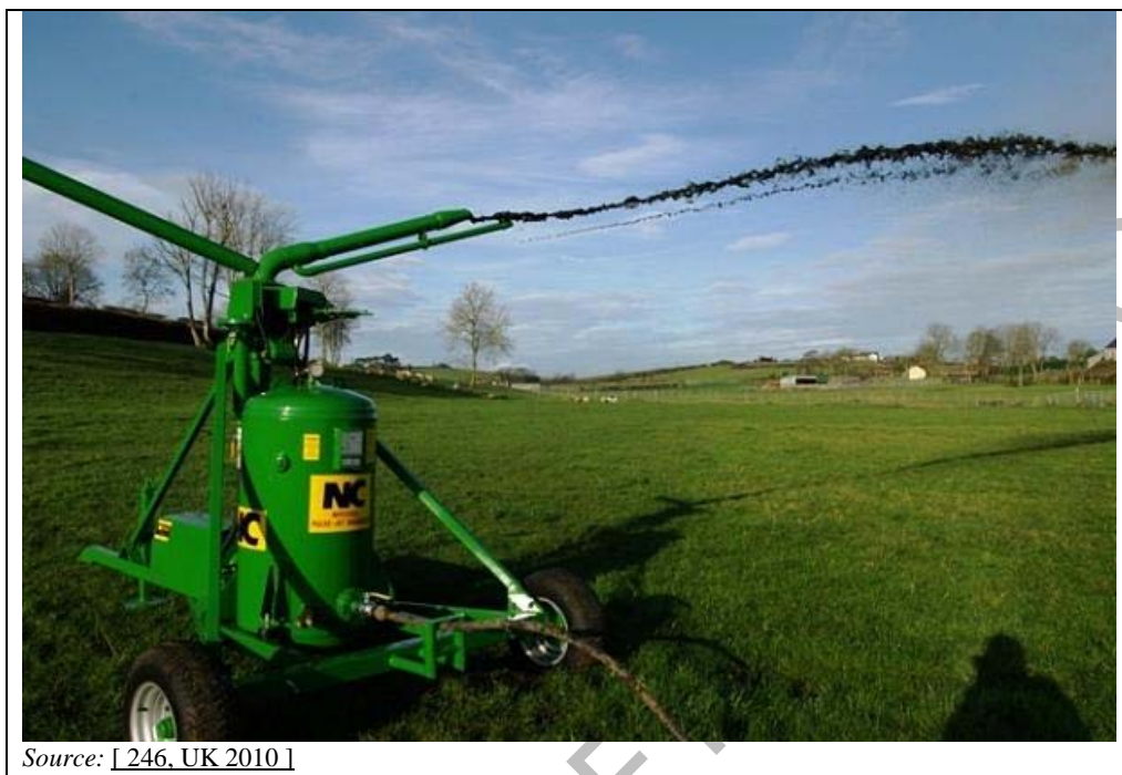
Figure 2.44: Pulse jet irrigator in operation
